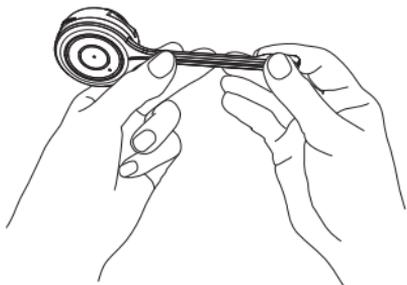
Holding the headset, rotate the headband to bring the boom close to your cheek.
