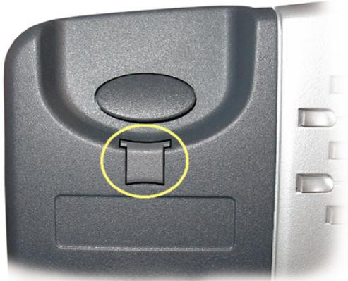
Install the handset retainer clip as shown below for wall mount use or high desktop positions, where the handset may be inadvertently bumped from the cradle. Pull out the clip as shown, rotate the clip 180°, and then re-insert the clip. The tab should protrude into the hookswitch area.
