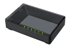
The Audiotrix C2 is a VoIP Analog Adaptor that interconnects analog telephones, faxes, and modems into SIP based systems. This ATA allows operators to shorten deployment time and ensure a highly secure environment to enable cloud telephony services into branch offices and SMBs.
