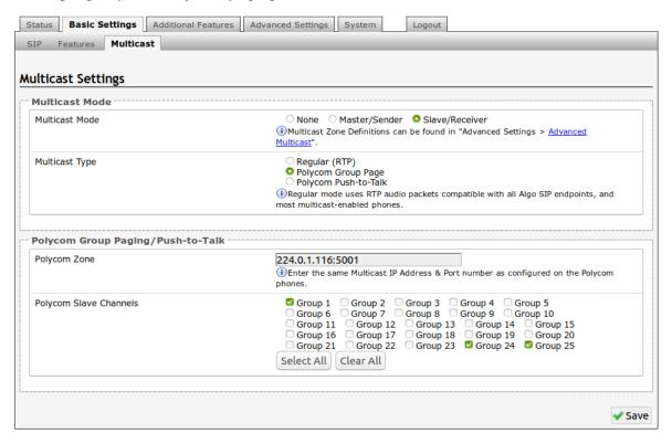
The Polycom phone used as page audio source for the 8186(s), must be configured to use either the G.711 or G.722 audio codec. The Polycom phone(s) must also be configured with the "Compatibility" setting ("ptt.compatibilityMode") disabled in order for this codec setting to be applied.
