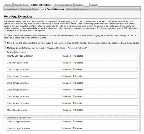
Additional SIP extensions can be registered for each multicast zone that will be used. This allows the advantage of dialing directly to a zone without needing to enter DTMF Codes (e.g. speed-dial keys can be used), but this may require additional SIP licenses depending on the SIP provider.
