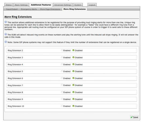
Up to 10 SIP Ring extensions can be registered. To configure additional ring extensions, click "Enable" beside the target extension and enter the Extension, Authentication ID, and Authentication password. A unique Ring Tone and multicast zone can be assigned to each extension if desired.
