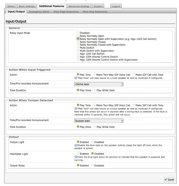
When triggered by an input relay, the 8186 SIP Horn Speaker can perform actions such as playing a pre-recorded announcement over the speaker(s), sending the announcement as a private message to a phone, or initiating a two-way conversation between the speaker and a phone.
