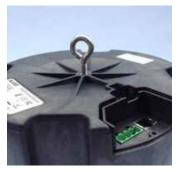
Heavy duty UL2043 compliant housing protects speaker and circuitry against dust and condensation. Integrated attachment for optional 1/4" 20 eye bolt ceiling suspension. RJ45 jack and IO Connector are hidden once installation is complete.
