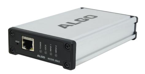
The Algo 8063 IP Door Controller is a compact and capable PoE powered digital IO interface designed specifically for door opening control and IP integration with legacy facility infrastructure.
