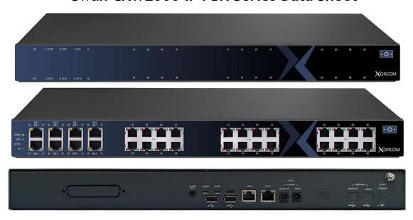
The Swan IP PBX series showcases Xorcom's CompletePBX distribution, offering support for FXS, FXO extensions and trunks. Swan can be outfitted with as many as 32 analog ports, and up to 2 E1/T1 PRI, T1 CAS, or E1 R2 ports, all contained within a compact, 19" 1U chassis. Additionally, it facilitates the integration of Astribank telephony interfaces and IP gateways. Supports 100-500 extensions (license-based), up to 200 concurrent calls.
