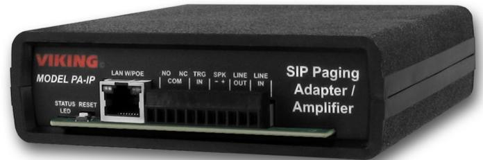
A built-in 6 Watt class D amplifier with speaker output connections are also provided to drive up to six analog speakers. A programmable relay output is provided for triggering external amplifiers, etc.
