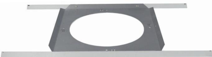
The **SA-TBA** is a tile bridge designed to mount 8 inch loud speaker and bridges both 2 ft x 2 ft and 2 ft x 4 ft ceiling tiles. It is compatible with the Viking models **SA-1S**, **30AE**, **35AE**, and **40AE** speakers. The **SA-TBA** tile bridge is constructed of 24 gauge cold rolled steel with an electro galvanized rust-resistant finish.
