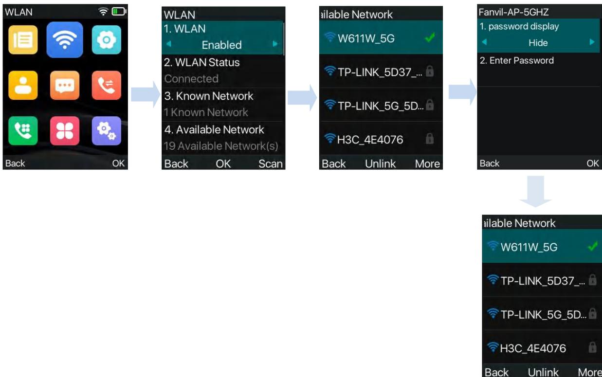
**Picture 6 - Wi-Fi connection on the device end**
