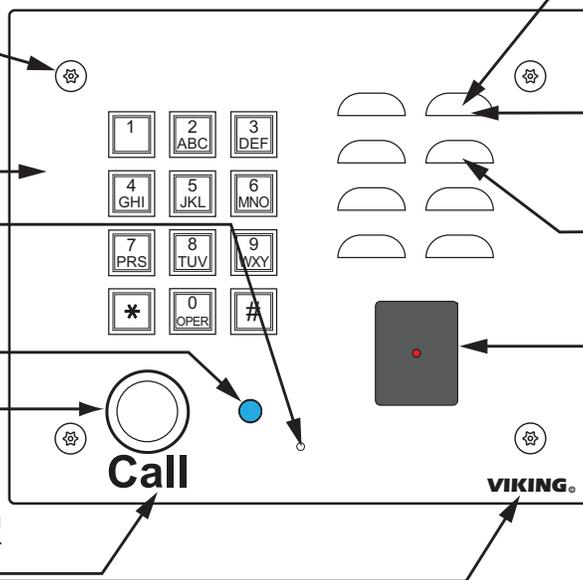
**Speaker:** Mylar speaker with rubber gasket to maintain water-tight seal and eliminate water deterioration.
