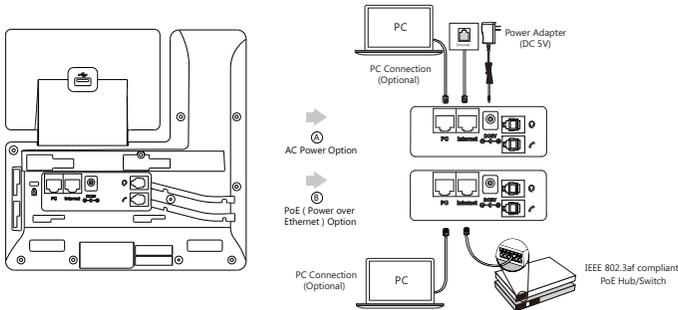
**Note:** The IP phone should be used with Yealink original power adapter (5V/2A) only. The use of the third-party power adapter may cause the damage to the phone. If you are connecting a PC to your phone, we recommend that you use the Ethernet cable provided by Yealink. If inline power (PoE) is provided, you don't need to connect the power adapter. Make sure the hub/switch is PoE-compliant.
