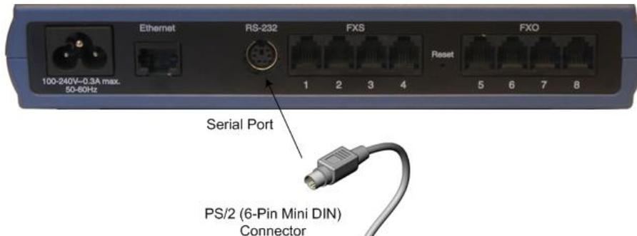
**Figure 2-7: MP-124 Serial Connection with PC for CLI Communication (e.g., MP-124 Rev. E)**
