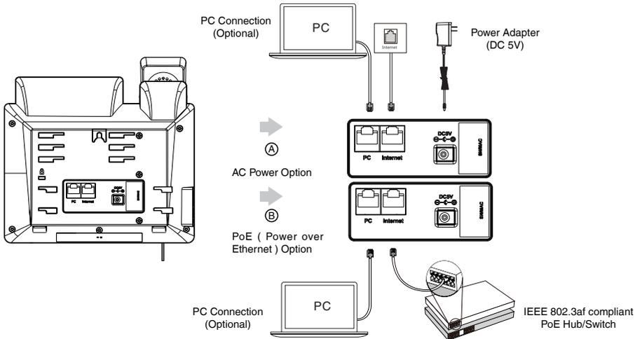
The IP phone should be used with Yealink original power adapter (5V/600mA) only. The use of the third-party power adapter may cause the damage to the phone. If you are connecting a PC to your phone, we recommend that you use the Ethernet cable provided by Yealink. If inline power (PoE) is provided, you don't need to connect the power adapter. Make sure the hub/switch is PoE-compliant.
