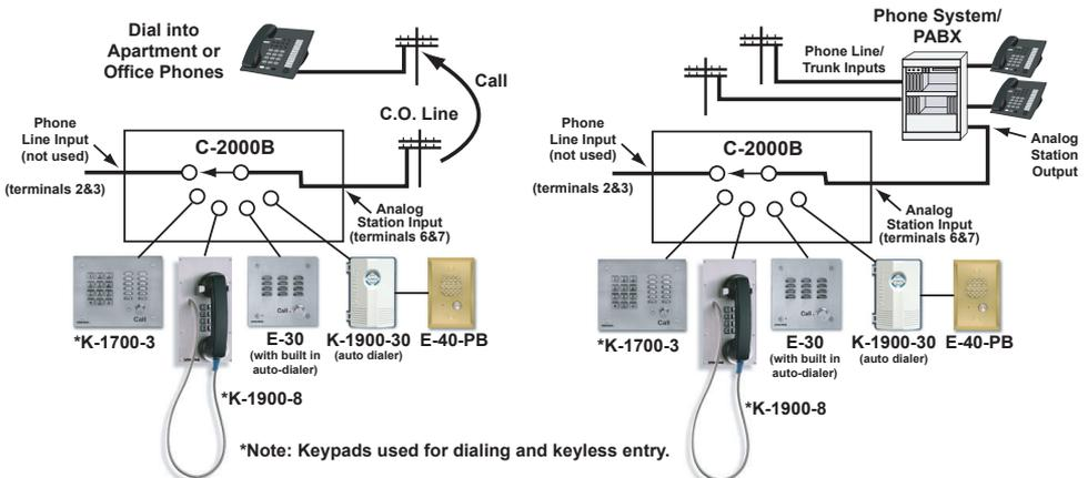
\***Note:** Keypads used for dialing and keyless entry.
