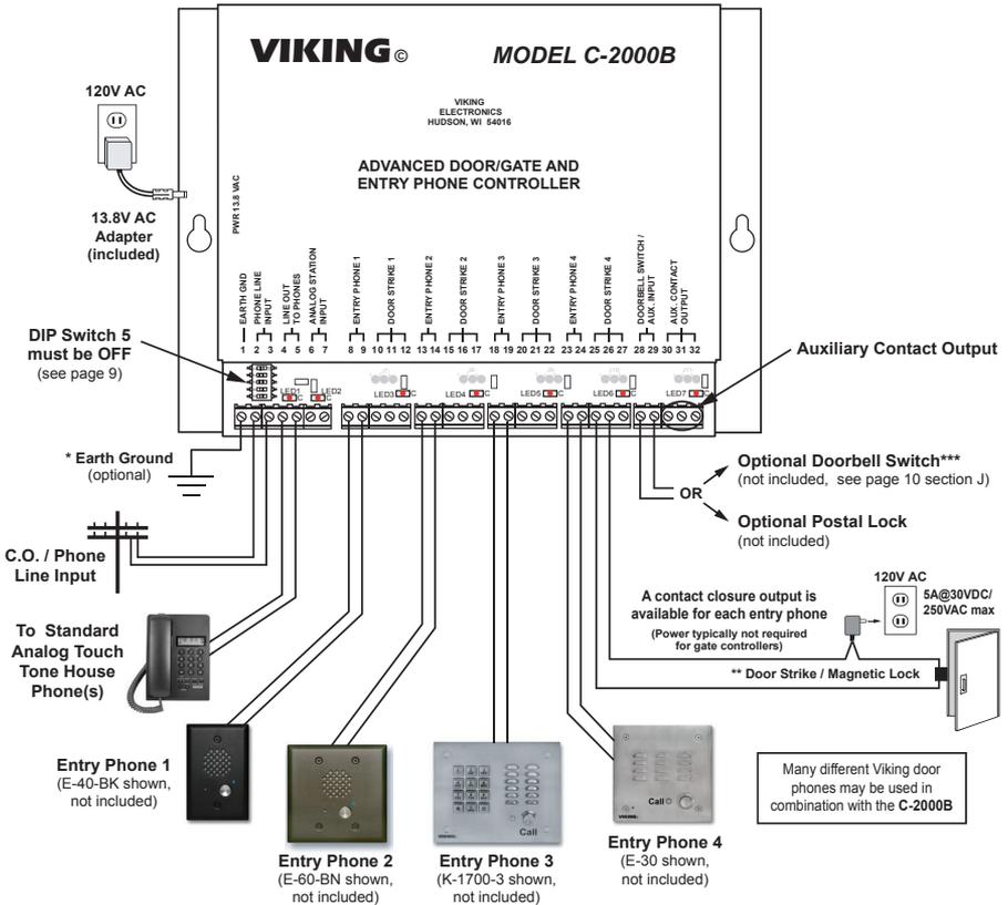
\***Note:** To increase surge protection, fasten a wire from the screw terminal to Earth Ground (grounding rod, water pipe, etc.)
