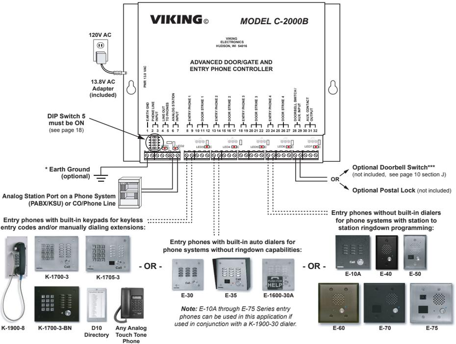
\* **Note:** To increase surge protection, fasten a wire from the screw terminal to Earth Ground (grounding rod, water pipe, etc.)
