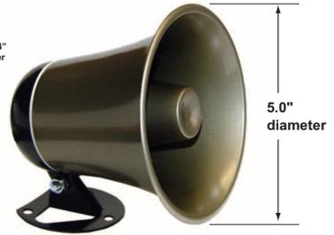
**Installation:** The **25AE** paging horn is designed to be surface mounted to any rigid surface. Designed to meet IP53 ingress protection rating when mounted with horn pointing downward at least 45 degrees from horizontal.
