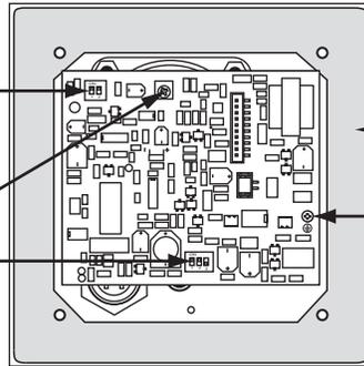
**Faceplate Gasket:** 1/8" thick closed cell PVC to provide a water-tight seal.
