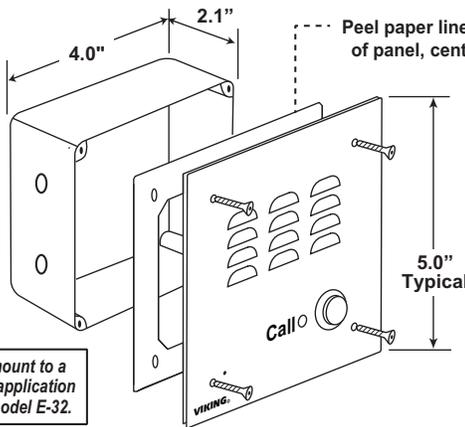
Peel paper liner and adhere gasket to back of panel, centering over mounting holes.
