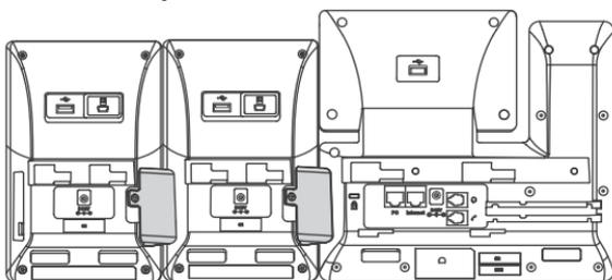
Note: The T53/T53W/T54W/T57W/T58A/T58A with camera IP phone can support 3 expansion modules at most. But if you use more than one expansion module, you need to connect an additional Yealink power adapter (5V/2A) to any one of the expansion modules. The power adapter should be purchased separately.
