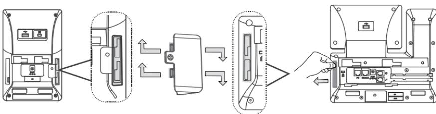
You may need to pull out the silica gel on the phone when connecting expansion module.
