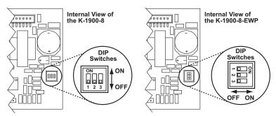
Note: DIP switch 3 is not used and should stay in the OFF position.
