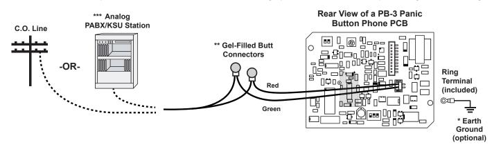
\* Note: To increase surge protection, loosen the PCB mounting screw labeled (as shown) and fasten a wire with ring terminal (included) from the mounting screw to Earth Ground (grounding rod, water pipe, etc.)
