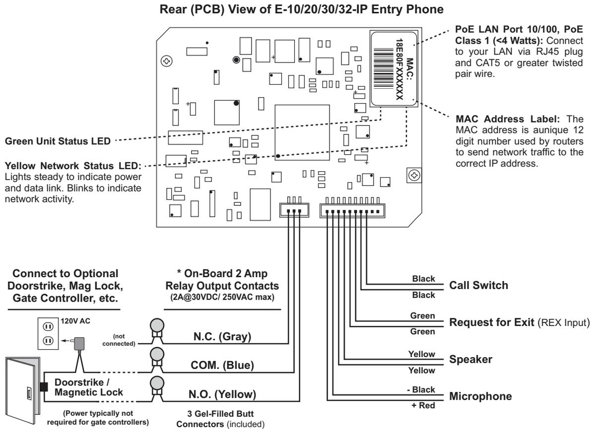
**Note:** The gel-filled (water-tight) butt connectors are designed for insulation displacement on 19-26 gauge wire with a maximum insulation of 0.082 inches. Cut off stripped wire ends before terminating.
