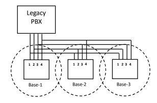
Re: when a call is coming in from L1, all handsets can pick up the call, as long as the handsets are in the coverage of base1~3.
