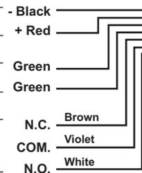
**Connect to Optional Doorstrike, Mag Lock, Gate Controller, etc.**
