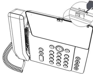
Picture 3 - Adjust shutter switch
