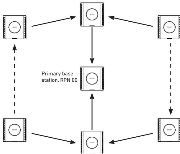
**Continuous line:** Shows the primary sync paths, with the relevant base stations chained in the multicell network.
