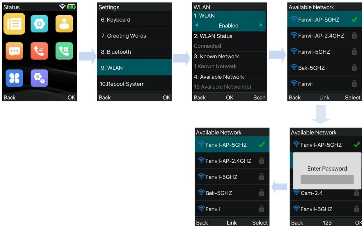
**Picture 6 - Wi-Fi connection on the device side**
