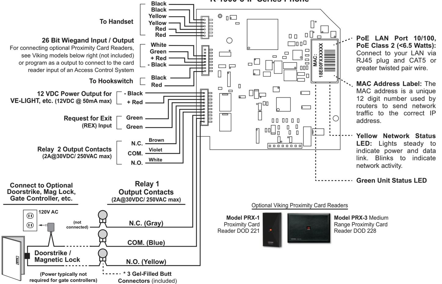
**Note:** The gel-filled (water-tight) butt connectors are designed for insulation displacement on 19-26 gauge wire with a maximum insulation of 0.082 inches.
