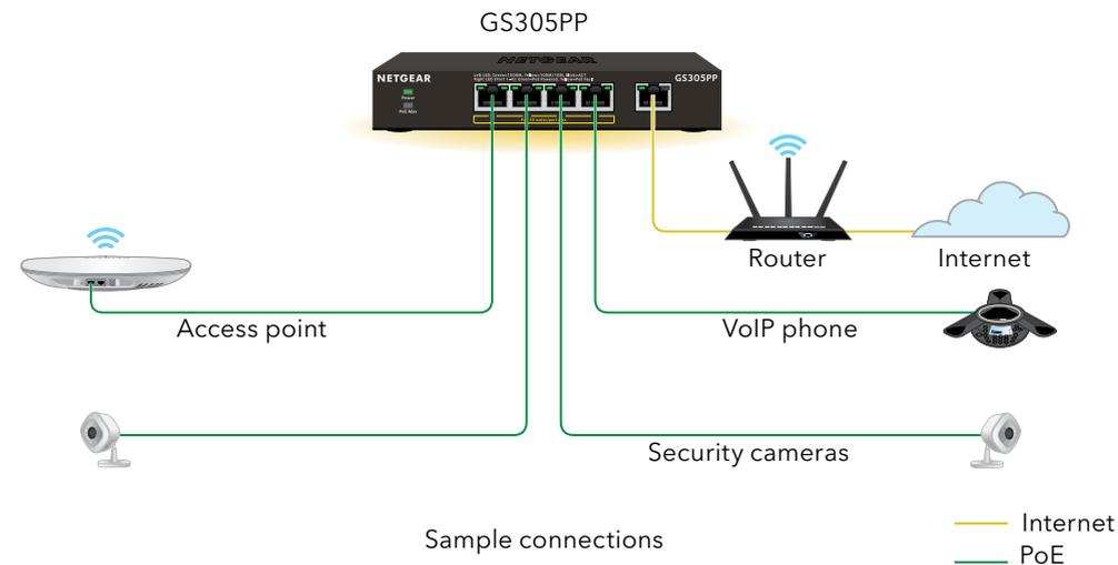
**Note:** The GS305PP switch supports both 802.3at (PoE+) and 802.3af (PoE). Model GS305P supports 802.3af (PoE) only.
