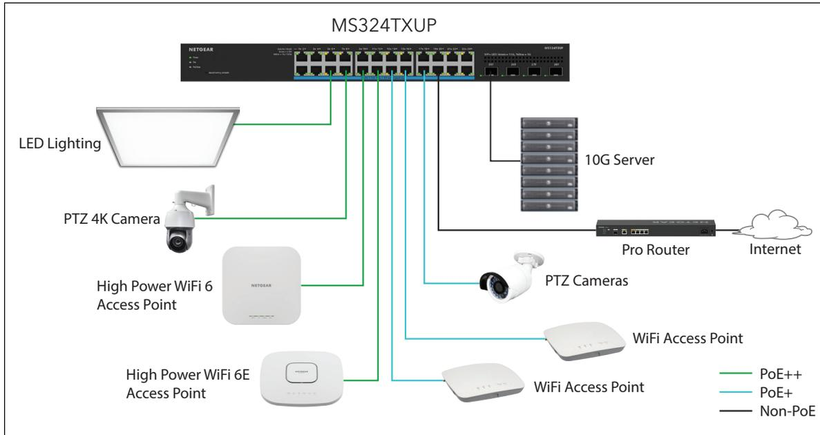
MS324TXUP Sample Connection Diagram
