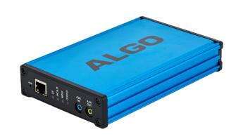
The 8300 IP Controller is an endpoint supervision tool designed for centralized device monitoring and management for Algo IP Endpoints. The 8300 provides system reliability for mission-critical voice paging / public address (PA) and emergency notification systems.
