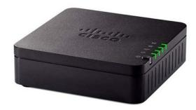
The Cisco ATA 191 Analog Telephone Adapter is a 2-port handset-to-Ethernet adapter that brings traditional analog telephony devices into the IP world.
