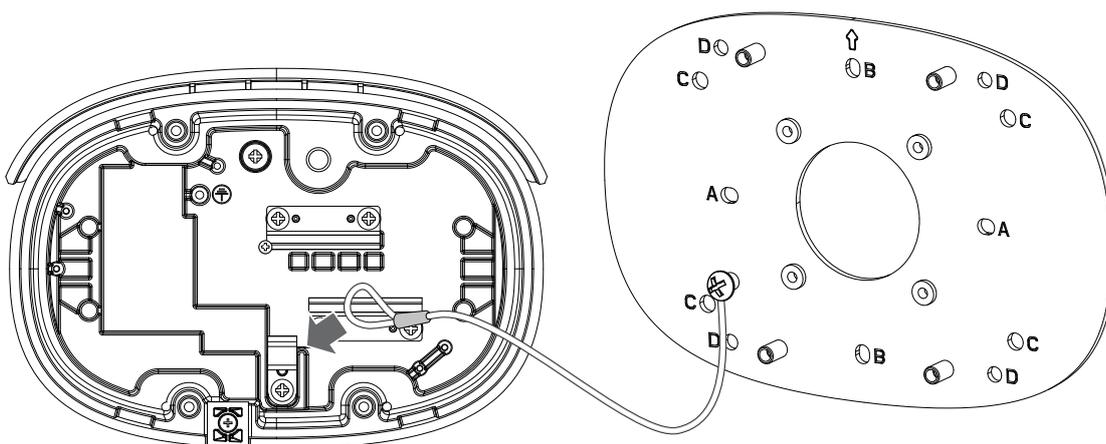
8. Align the camera with the mounting plate, and then secure the T10 anti-tamper screws to install the camera.
