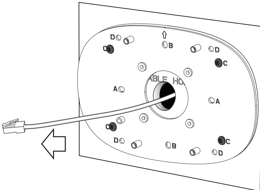
5. Pass an Ethernet cable through the waterproof cable gland components, and through the rubber seal as shown below. Connect the Ethernet cable to the camera's RJ45 onnector. Tighten the components to prevent water ingress.
