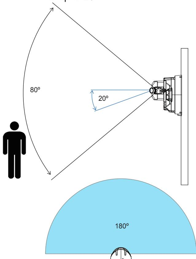
The field of view is illustrated on the left. Note that the higher the camera is installed, the larger is the blind spot area underneath the camera. The camera can be mounted at a height of 3 meters to cover a panoramic view area with its center of view aiming at the horizon.
