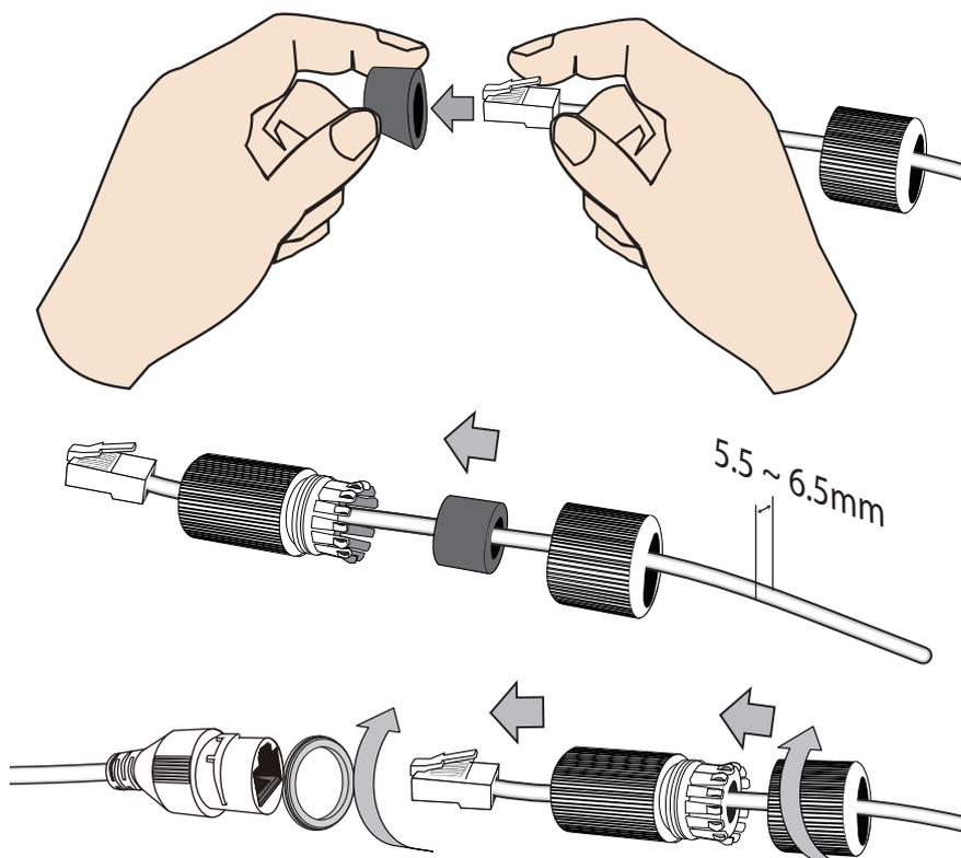
5. Press the Ethernet waterproof enclosure in between the retention clips at the back of the camera. The retention clips will hold the enclosure in place. Connect the ground wire to a grounded earth rod with a resistance smaller than  $4\Omega$ , with a section area larger than  $25\text{mm}^2$ , to a ground rod 1.5 meters into the ground.
