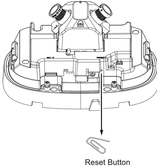
The reset button is used to reset the system or restore the factory default settings. Sometimes resetting the system can return the camera to normal operation. If the system problems remain after reset, restore the factory settings and install again.
