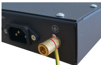
Figure 3. SIP/E1 Gateway – Grounding device
