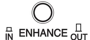
The rear panel AE adjustment controls the mix of the Audio Enhancement effect with the audio signal. Counterclockwise rotation of the control minimizes the Audio Enhancement effect. Clockwise rotation of the control maximizes the Audio Enhancement effect.
