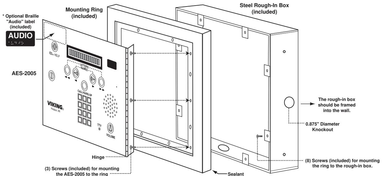
**Important:** If the enclosure is to be mounted outdoors, use an appropriate sealant around the outer edge of the mounting ring.
