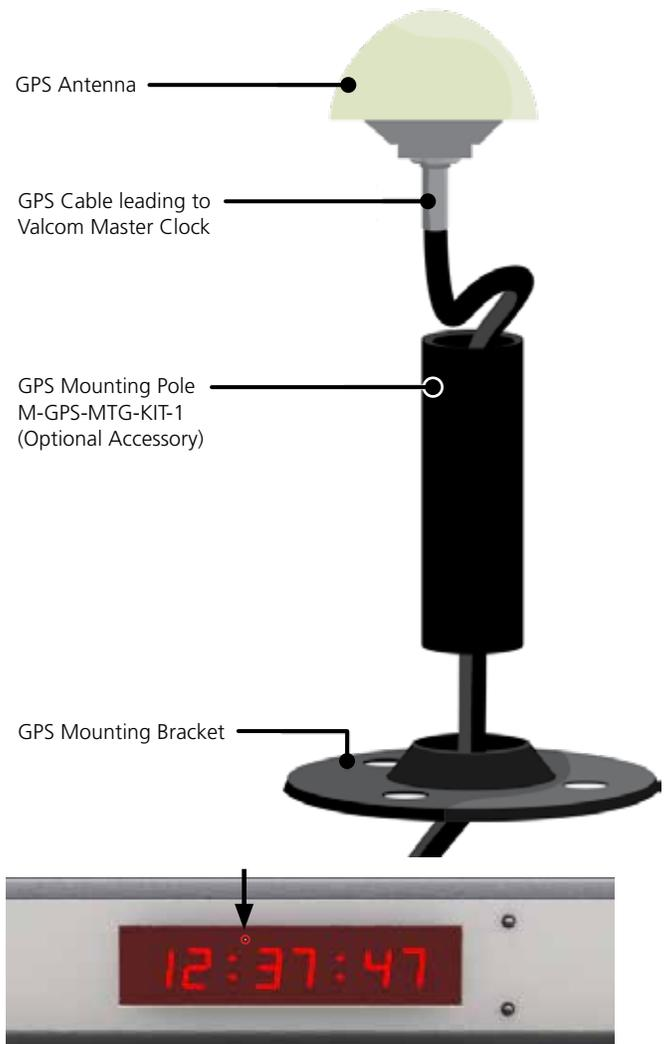
If your master clock is set to receive GPS time data as its primary time input, a loss of GPS time data will cause a red blinking circle to appear above and to the left of the third digit on the LED time display.
