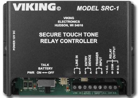
The **SRC-1** also provides up to 32 (1 to 6 digit) programmable keyless entry codes to operate the relay from the entry phone. Keyless entry can be disabled in programming for increased security.
