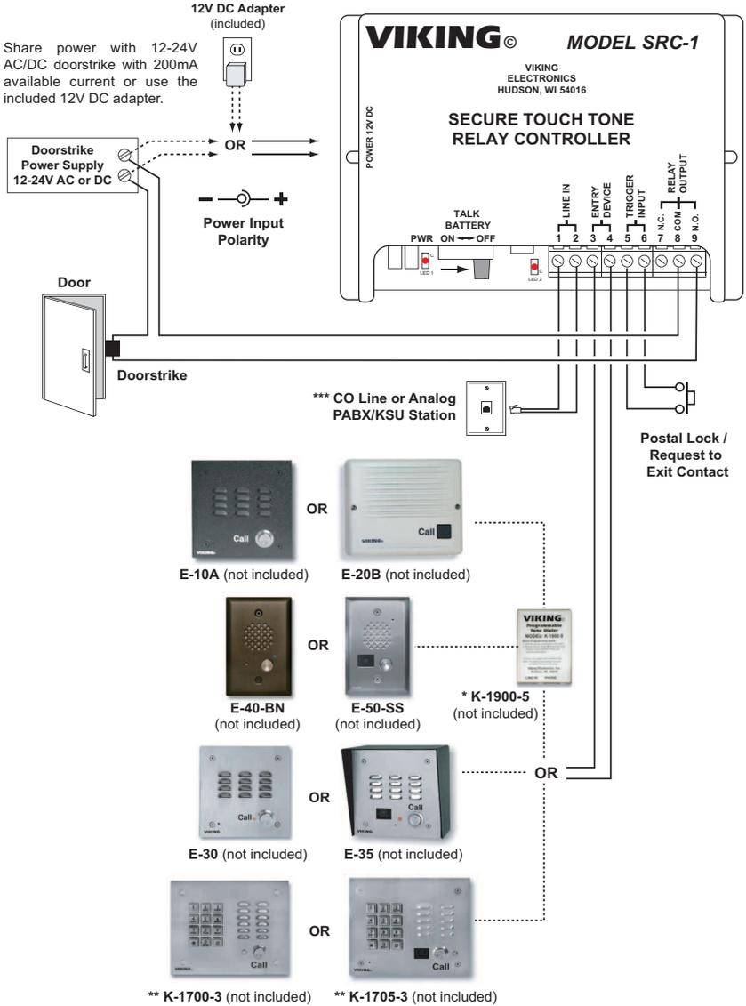
\* **Note:** The K-1900-5 Dialer is not required if installed on a ringdown circuit. The K-1900-5's touch tone and flash restrictions must be disabled (\*02).
