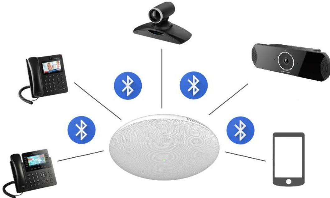
Figure 24: Connecting the GSC3510/GSC3505 as a Bluetooth Speaker
