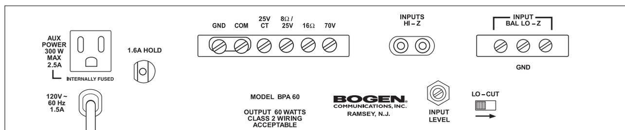
Fig. 1 - BPA60 Rear Panel Connection Diagram
