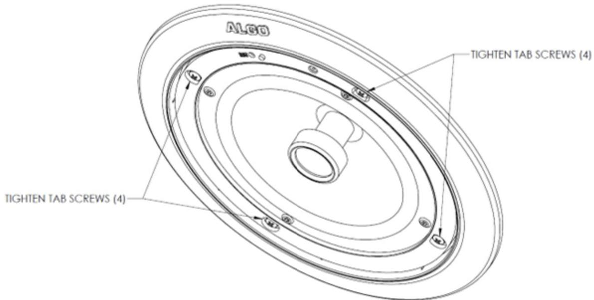
2. After installation and testing, gently work the speaker grill into its friction fit position and ensure it is evenly flush with the housing around the edge. The speaker grill is intentionally tight to prevent falling from the ceiling.
